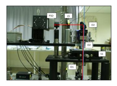
Figure 1. Cobolt Rumba™ 1064 nm in a steerable laser trap, stage and detection assembly. (Co of Terence Strick).
