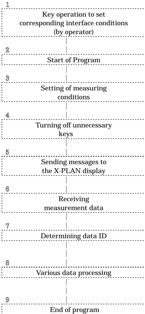
First the interface conditions are set by manual operation.(At least the starting baud rates should correspond with each other.)
